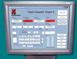
Communications paths are controlled by the console operator and each radio user can talk with the operator on demand. This solution supports multiple operator positions and channels.
